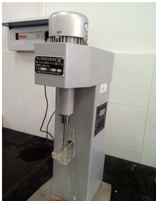
Fig. 3. XFG flotation machine for pure mineral flotation tests.
